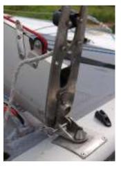
**7.** Walk the mast up from the stern, you will need to step onto the trap or pass the mast to a 3<sup>rd</sup> person already on the deck to complete this. At the same time the 2nd person should be pulling the mast up using one of the trapeze wires.
