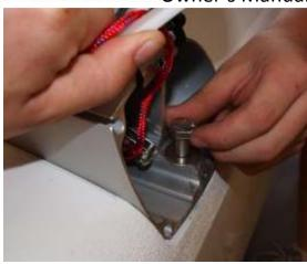
Wipe all dirt and grease from the beam pad before sitting the beam on. Make sure the beams are facing the correct way. The rear beam should have the traveler saddles facing backwards. Apply grease to the threaded part of all bolts before inserting them into the hull. Get all the bolts started before tightening any of the bolts. We recommend beginning with the inner front beam bolt. If a particular bolt is being difficult to fit. Release all the beam bolts and fit this bolt first.
