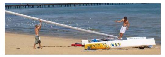
**8.** When the mast is vertical allow the mast to rotate so that sail groove now faces backwards. **DO NOT** let the mast rotate until it is vertical.
