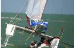
As soon as the boat is upright, grab the dolphin striker. This will, not only keep the boat from capsizing to the other side, but will also keep you and the crew connected to the boat. Climb aboard over the front beam and use the dolphin striker as a step.
