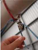
**2.** Take the Dyneema end and tie it to the mast spanner and cleat the other end into the hoisting cleat, this will stop it falling out while raising the mast.
