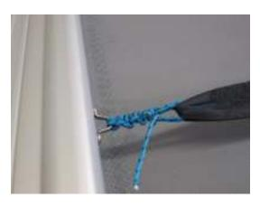
**14.** Remove the bottom half of the Stamasters from the side stays and attach to the side chain plates with the locknut on the inside and the control line loop facing forward.
