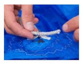
**4.** The spinnaker sheets are attached by hitching the red connecting loop in the middle of the spinnaker sheet though the eyelet in the clew of the spinnaker.
