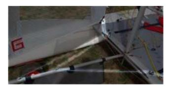
Pass the jib traveler line (red) trough the saddle on the spinnaker pole and then cleat it off in the cleat on the beam.
