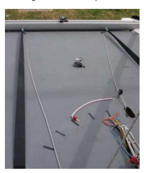
2. Pass the retrieval line trough the eyelet in the bottom of the chute and use the tiller extension to pull it up and out by poking the extension down and tying the line to it.
