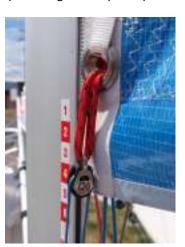
The clip on the end of the downhaul rope hooks into the hole the mast spanner.
